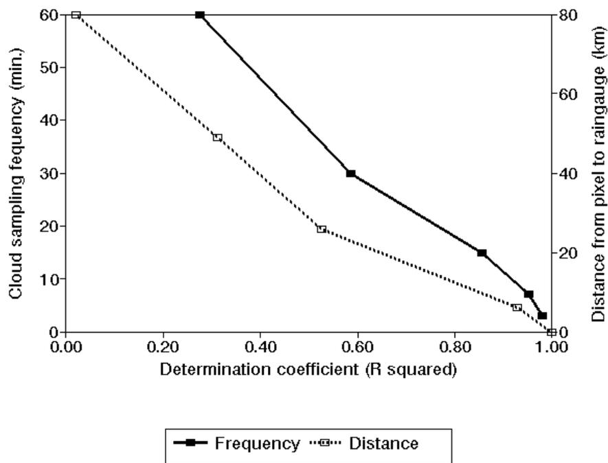
**Figure A2: correlation (measured as the coefficient of determination, abscissa) between simulated average dekad pixel rainfall and (i) a distant raingauge (km, dotted curve, right axis), (ii) cold cloud duration over the pixel sampled at different intervals (minutes, solid curve, left axis). The figure is based on a simulation covering 500 days accumulated into 50 10-day periods.**
