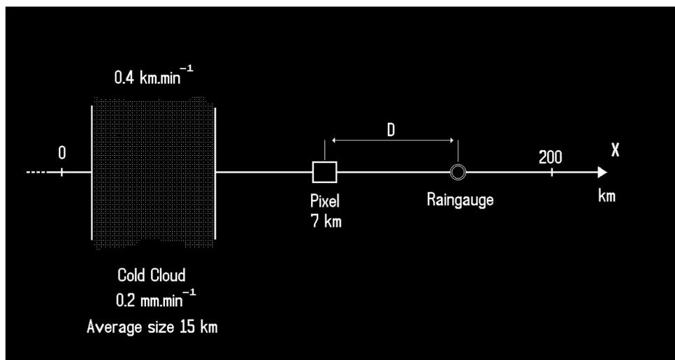
**Figure A1: a simple one-dimensional model of rain-bearing cloud, pixel and raingauge. Refer to the text for details.**
