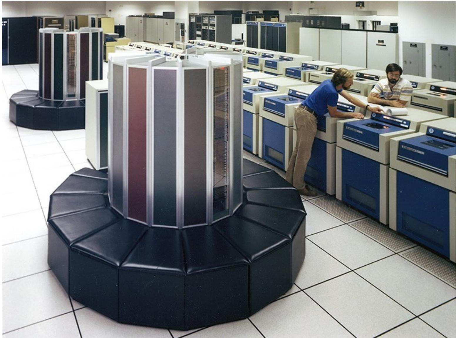
*Cray-1 supercomputer: before the BLAS programming tool was introduced in 1979, there was no linear algebra standard for researchers working on machines such as the Cray-1 supercomputer at Lawrence Livermore National Laboratory in California. Credit: Science History Images/Alamy*
