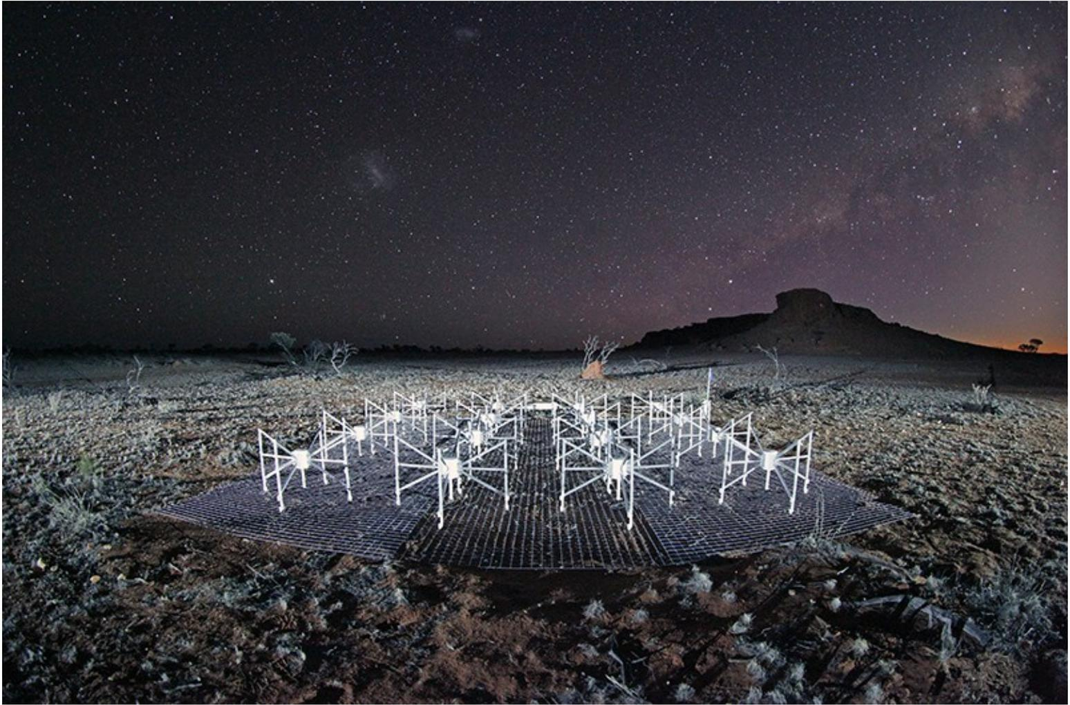
*A night view of part of the Murchison Widefield Array, a radio telescope in Western Australia that uses fast Fourier transforms for data collection. Credit: John Goldsmith/Celestial Visions*
